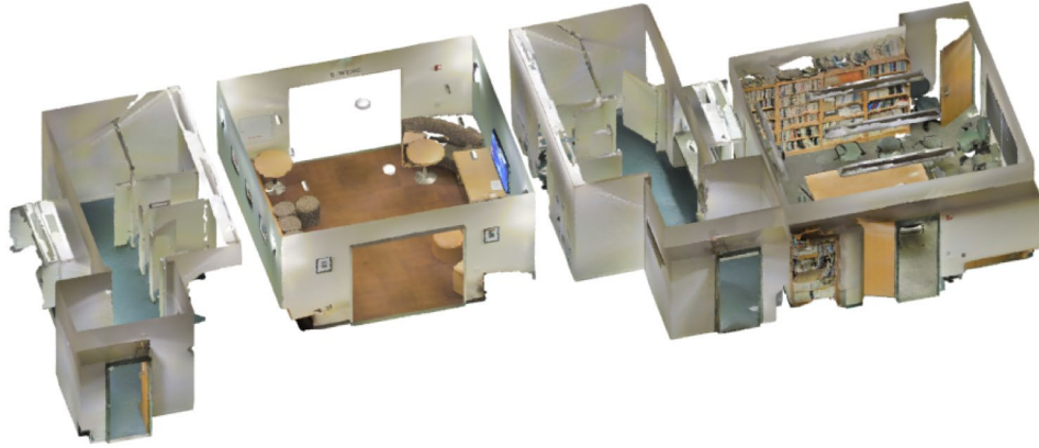
scanned point cloud
