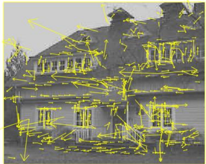
Figure 5: This figure shows the stages of keypoint selection. (a) The 233x189 pixel original image. (b) The initial 832 keypoints locations at maxima and minima of the difference-of-Gaussian function. Keypoints are displayed as vectors indicating scale, orientation, and location. (c) After applying a threshold on minimum contrast, 729 keypoints remain. (d) The final 536 keypoints that remain following an additional threshold on ratio of principal curvatures. Figure from [Lowe 2004]
