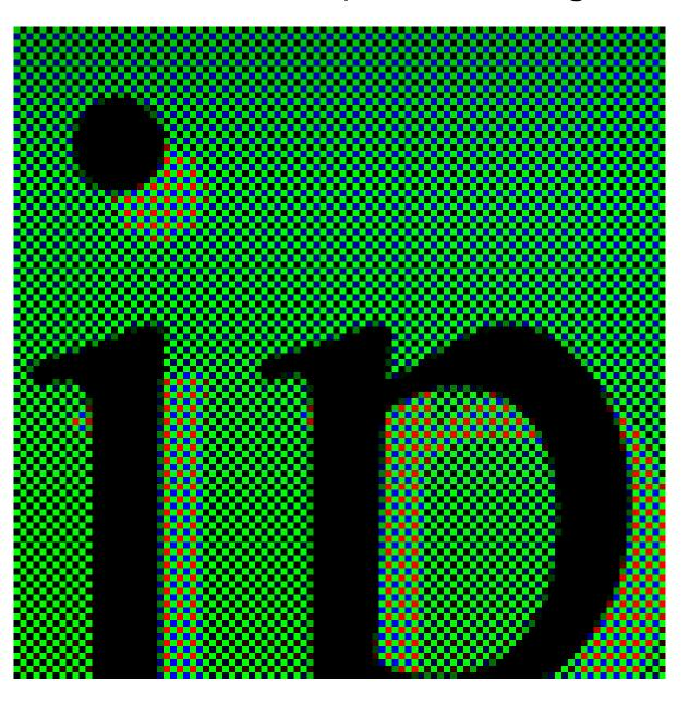
Every pixel of the array is only sensitive to a single colour.
