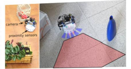
Fig. 1. The Mighty Thymio robot in two environments: five proximity sensors can easily detect obstacles at very close range (blue areas), whereas the camera has a much longer range (red area) but its outputs are hard to interpret.
