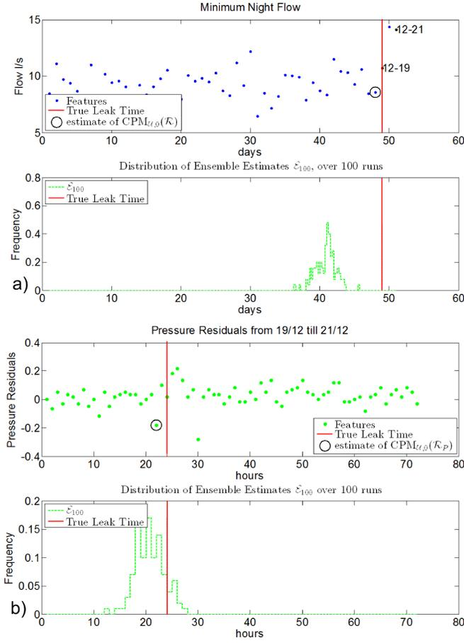
**Fig. 3.** Analysis of the minimum night flow to estimate the time instant when a leakage appeared in the network. The leakage occurred at 20<sup>th</sup> of December and lasted for two days.
