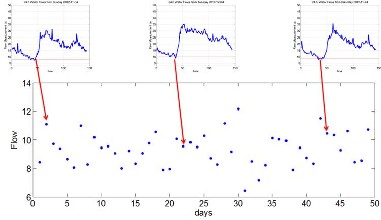
**Fig. 1.** An illustrative example of the sequence  $\Phi$ . The values of  $\Phi$  are displayed in the plot below, and correspond to the minimum night flow of each specific day. The small plots above represent the daily flows: the value of the minimum night flow is plot as an horizontal (red) line.
