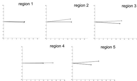
Figure 12: Displacement vectors  $\vec{v}$  estimated in camera images. In each plot, the solid line indicates the true displacement vector obtained by matching corners of pictures at initial and final camera position. Dotted line represents the estimated displacement vector  $\vec{v}$ .
